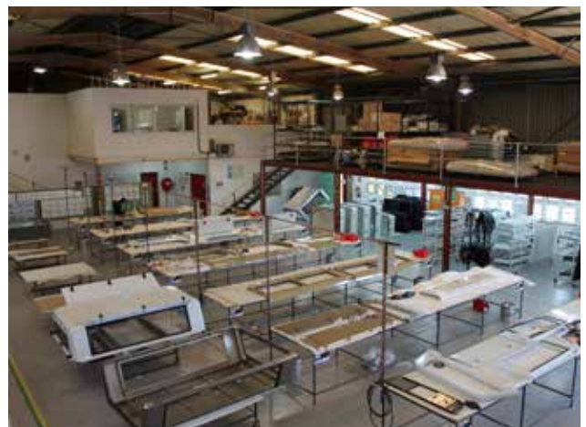
RSI has now developed a patent-pending modular design to construct their canopies. Instead of a single welded unit, the canopies are made up of five key components: roof, two side panels, the front panel and rear door.
